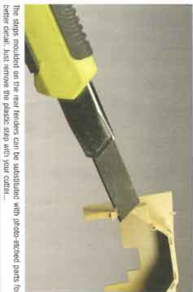
The steps moulded on the rear fenders can be substituted with photo-etched parts for better detail. Just remove the plastic step with your cutter...
